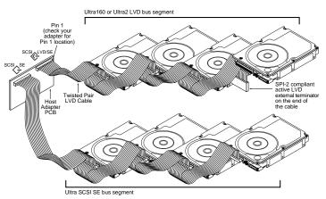
Figure 3. Cable connections and external termination
